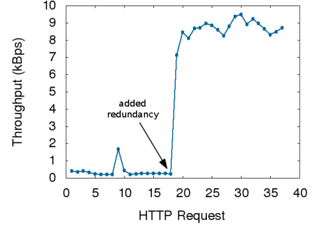
Fig. 6. Throughput before and after handover.
