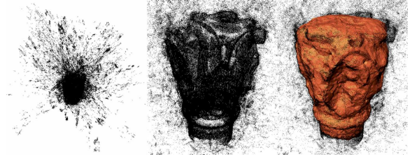
Figure 10: The point cloud on the left was captured via multi-view stereo – note the substantial structured outliers. The center image is a zoomed-in portion of the point cloud, centered on the object of interest. The method of [GCSA13] (right) is highly robust to outliers, while still preserving the details of the object, due to the use of parity and an unsigned distance function which adapts to the noise.
