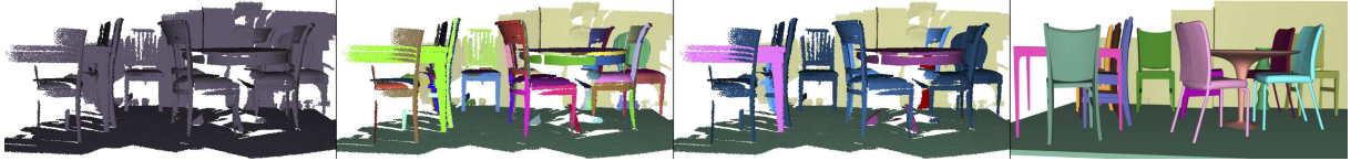
Figure 15: From the incomplete and cluttered scan on the left, the approach of [NXS12] first oversegments the point cloud (mid-left), then iteratively merges segments which agree on class labels (mid-right), and finally deforms a set of detected models to best resemble their segmented objects (right).
