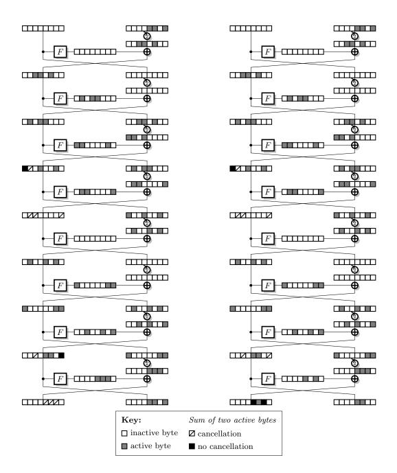
Fig. 2. Truncated characteristic for LAC with 35 active S-boxes.
