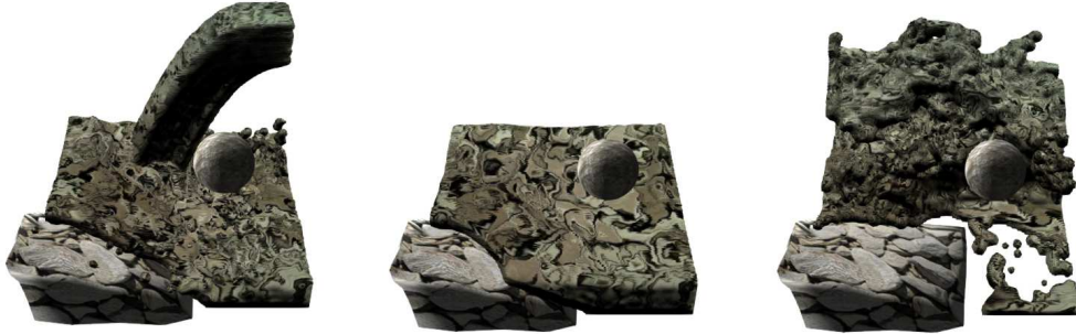
Figure 3: A 3D liquid simulation with obstacles in the domain implemented using the rasterization pipeline. The simulation runs at 35 FPS using 125k particles on a Quadro 2000M graphics card.
