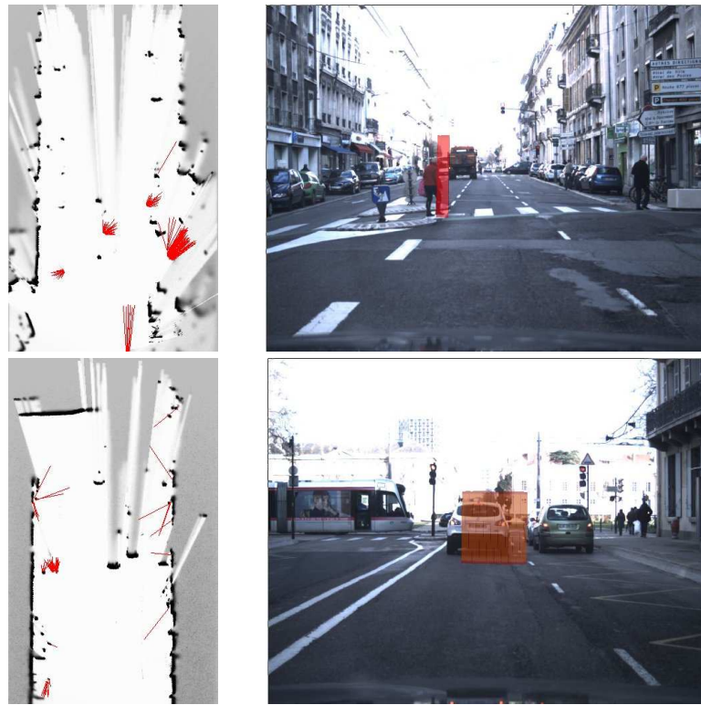
Fig. 9. First HSBOF and risk estimation results. Left image: output of the HSBOF process with the filtered occupancy grid (white for empty space, black for occupied space) and the velocity field (from each moving cell are drawn red rays representing the velocities). Right image: dangerous cells are reprojected in the camera image.
