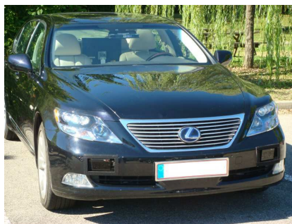
Fig. 4. Experimental platform : Lexus LS600h car equipped with two Ibeo Lux Lidars and cameras.
