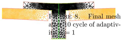
FIGURE 8. Final mesh after 10 cycle of adaptivity  $\alpha = 1$
