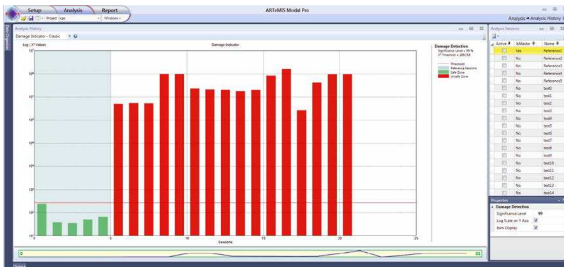
Figure 5. Example of damage control chart based on proposed subspace damage detection method.
