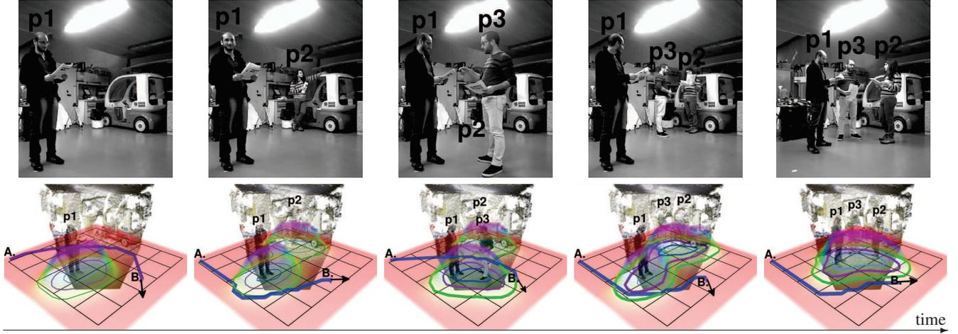
Fig. 6. Mapping the social interactions of three participants using the proposed approach along various time frames. The overlaid path plan between points **A** and **B** corresponds to the trajectory which best prioritises the regressed global social sensitivity.
