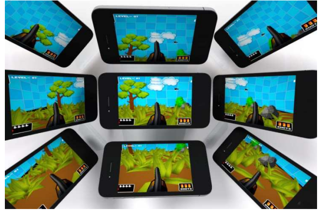
Figure 2: Tilt control: device orientation is applied to the camera.
