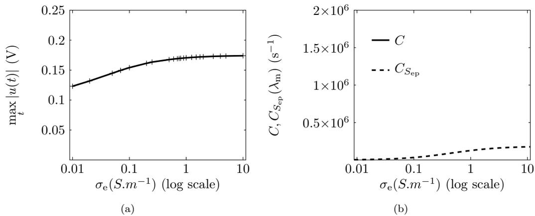
Figure 5: 5(a): Maximum  $\Delta$ TMP during simulations for the  $\beta$  (solid) and  $\lambda^2$  (dashed) static models. 5(b): Comparison of simulated and estimated Lipschitz constants  $C_{S_{ep}}$  for the  $\beta$  model. Solid lines : difference between non-linear and linear decay rates. Dashed lines : estimations from eq (30) with  $\lambda_m$  from figure 5(a).
