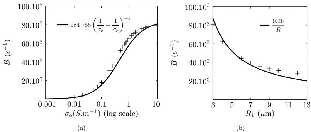
Figure 3: Linear conductivity model : evaluated decay rate  $B$  of the  $L^2$  error depending on the extracellular conductivity  $\sigma_e$  with  $R_1 = 6 \mu\text{m}$  (3(a)) and depending on the radius of the cell  $R_1$  with  $\sigma_e = 0.5 \text{ S/m}$  (3(b)). The first fitting constant has the same order of magnitude as  $R_1^{-1} \sim 167\,000$ . The other constant is of the order of  $(\sigma_e^{-1} + \sigma_c^{-1})^{-1} \sim 0.24$ .
