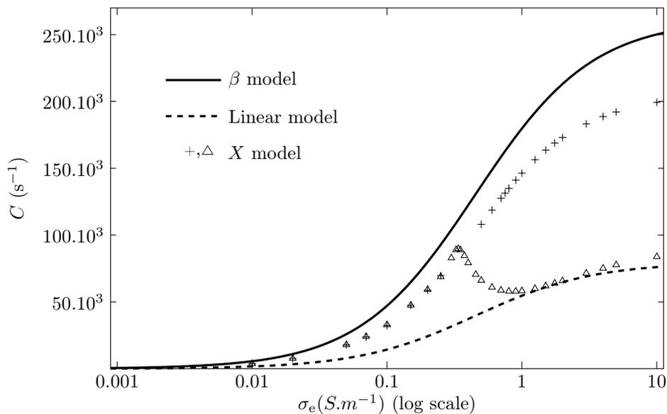
Figure 6: Decay rate to the periodic solution for the dynamical case  $S_m(\lambda) = S_0 + S_1 X(t)$ , compared to the evaluations already performed for the linear and the  $\beta$  models. Simulations of the dynamical model were made for several characteristic durations:  $\tau_{ep} = 1 \mu s$  (+),  $\tau_{ep} = 10 \mu s$  ( $\Delta$ ).
