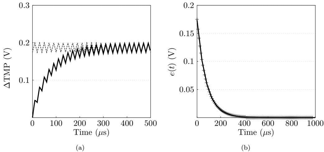
Figure 2: 2(a) : Transmembrane potential difference (solid) and periodic solution (dotted) of the linear problem, with  $\sigma_e = 0.2 \text{ S.m}^{-1}$ . 2(b) : Fit of the  $L^2$  error  $e(t)$  between the  $\Delta\text{TMP}$  and the periodic solution, giving the constant  $C_A$ .
