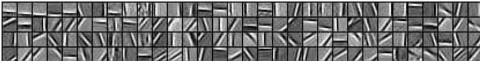
Figure 3: Filters obtained by the first layer of the convolutional kernel network on natural images.
