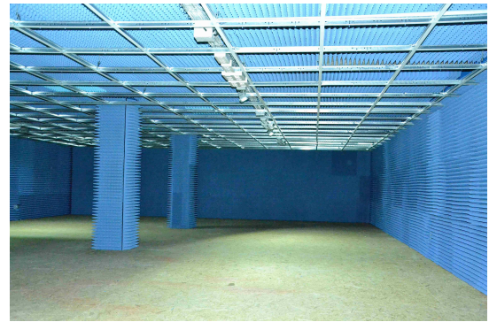
Fig. 2: Current status of FIT/CortexLab room, SDR platform will be attached to the roof, the room will have now 50 dB isolation so as to provide a reproducible experimental environment.
