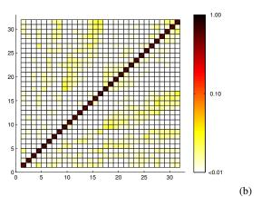
Figure 2: Inter-state(a) and intra-state(b) mixture transition matrices, averaged over states for CHiME data
