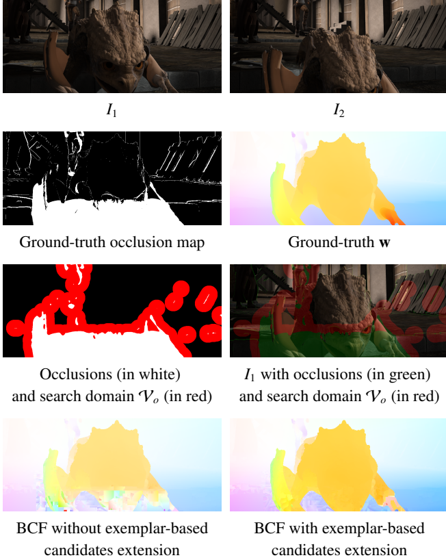
Figure 2: Illustration of the performance improvement with exemplar-based candidates extension (without the dominant motion extension). First row: two successive input images. Second row: ground-truth occlusion map and motion field. Third row: representation of the search domain \mathcal{V}_o (displayed here after median filtering of the occlusion map for the sake of visibility only). Fourth row: Best Candidate Flow obtained respectively without and with the exemplar-based candidates extension.
