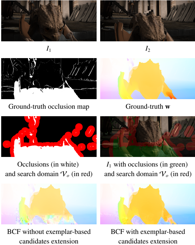
Figure 2: Illustration of the performance improvement with exemplar-based candidates extension (without the dominant motion extension). First row: two successive input images. Second row: ground-truth occlusion map and motion field. Third row: representation of the search domain \mathcal{V}_o (displayed here after median filtering of the occlusion map for the sake of visibility only). Fourth row: Best Candidate Flow obtained respectively without and with the exemplar-based candidates extension.
