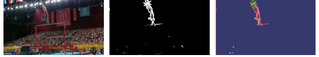
Figure 4. The original frame, its IME map and the result after segmentation are shown from left to right.
