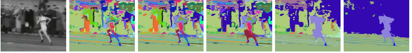
Figure 3. Example from action ‘Running’: The first two images depict a video frame and the initial super-voxel segmentation used as input of our approach. The four other images represent the segmentation after a varying number of merge operations.
