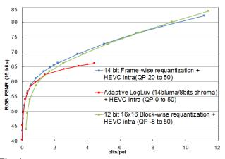
**Fig. 4**. Comparison between 14 bit frame-wise, 10 bit block-wise and frame adaptive LogLuv in [7].
