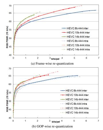
**Fig. 5.** Rate-distortion curves for HEVC intra and inter (QP 0-50) after : frame-wise method (a) and GOP-wise method (b).
