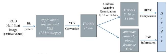
Fig. 1. Our general coding scheme for floating point HDR image encoding.
