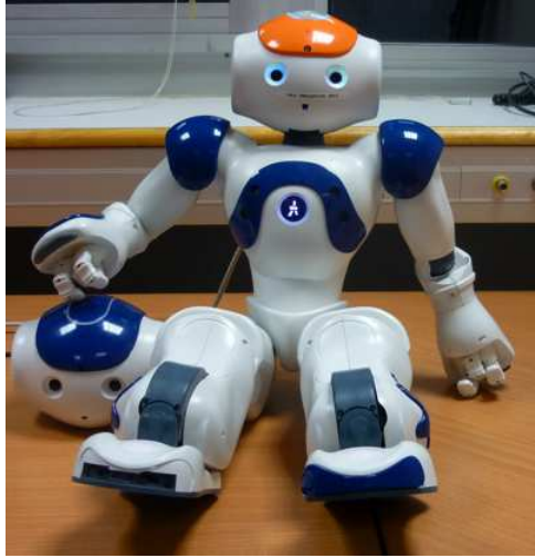
Figure 4: Within this work we use a prototype audiovisual head that embeds a binocular and synchronized camera pair, as well as two microphones. The “orange” head, used instead of the standard “blue” head, is fully interfaced by the RSB middleware described in this section.
