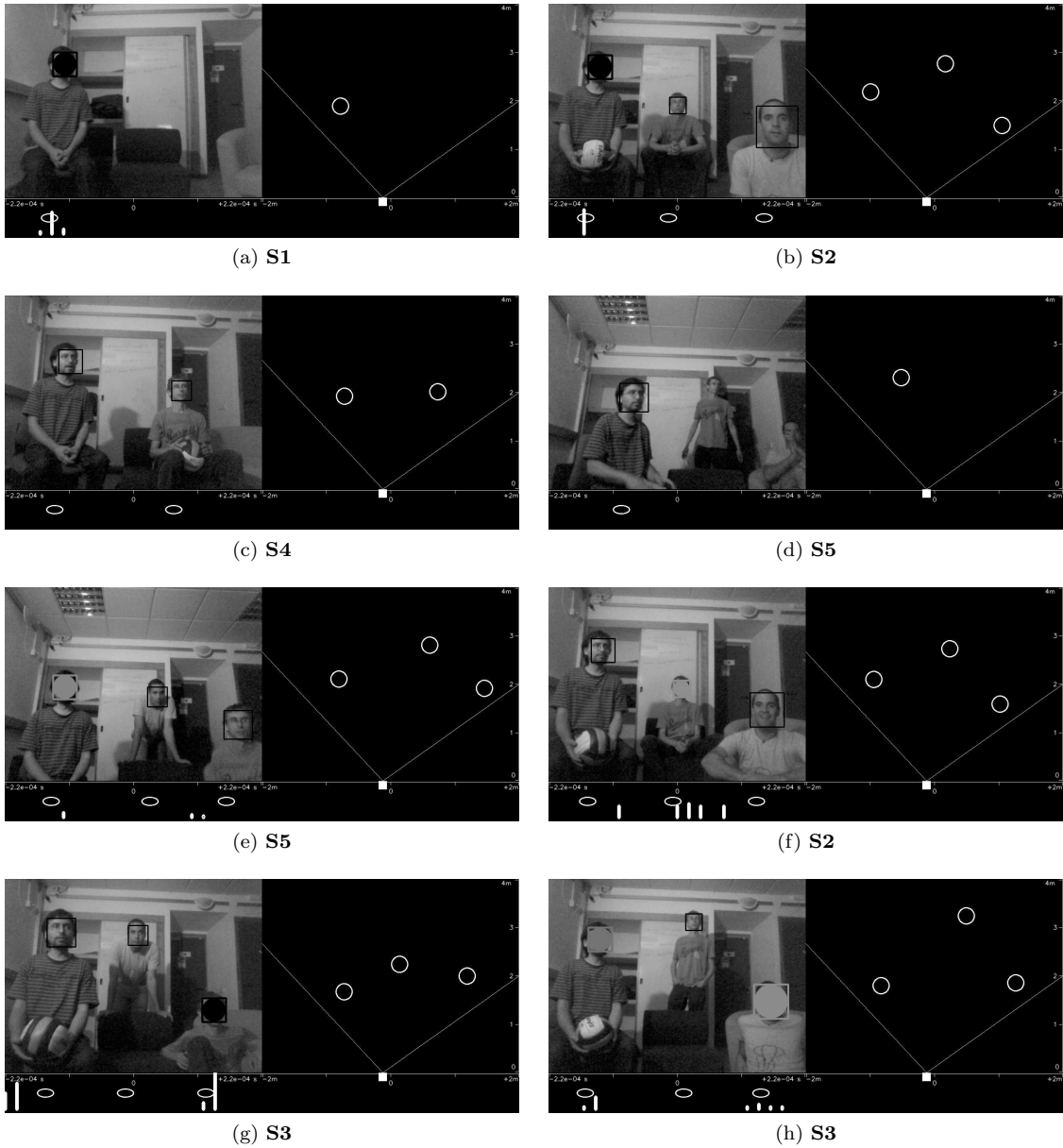
Figure 10: Snapshots of the visualization tool. Frames selected among the five scenarios to show the method's strengths and weaknesses. The faces' bounding box are shown superposed to the original image (top-left). The bird-view of the scene is shown in the top-right part of each subimage. The histogram of ITD values as well as the projected faces are shown in the bottom-left. See Section 7.3 for how to interpret the images above.
