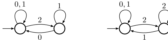
Fig. 5: Finite automata for the G^2 -shift (left) and for the (-G^2) -shift (right)
