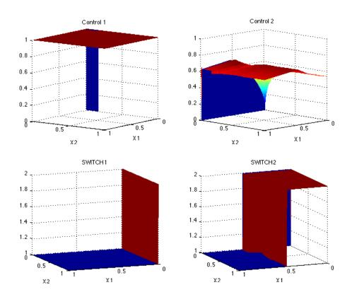
Figure 4: Example 5.3: control variables for electric engine (q = 1, left) and thermic engine (q = 2, right). Optimal feedback (upper) and optimal switching (lower).
