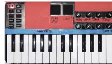
Figure 2: MIDI keyboard for playing the harmonizer (in red) and the synthesizer (in blue).
