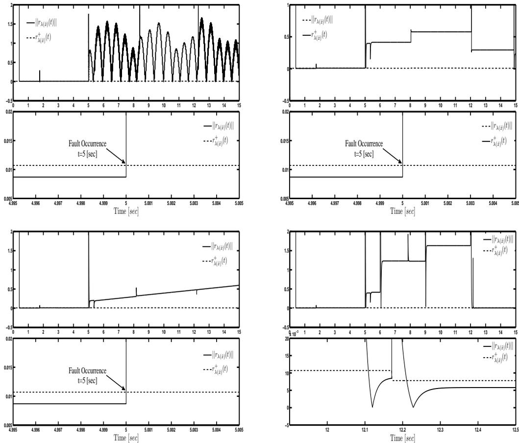
Figure 8. Fault Detection Decision. Faulty case. Notice that, in the intermittent fault, when the fault disappears,  $\|r_{\lambda(\hat{x})}(t)\|$  remains less than the threshold  $r_{\lambda(\hat{x})}^+(t)$  indicating that fault is already not present.
