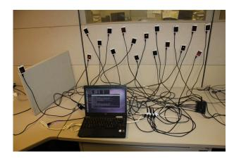
Fig. 4. Testbench with 18 energy-harvested ST GreenNet nodes in Crolles, France. 16 nodes are CoAP clients and one node is the CoAP server. The node on the far left is the PAN coordinator in the 802.15.4 beacon-enabled network. Nodes are connected to USB for the collection of experiment traces.
