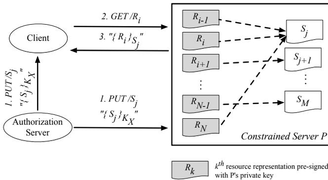
Fig. 2. Coupling OSCAR with the RESTful architecture of CoAP. Note that server-side digital signing operations are performed offline.  $\{X\}_K$  denotes the online symmetric encryption of  $X$  with the key derived from  $K$ . Encryption key  $K_X$  of a new access secret may depend on the key management scheme.
