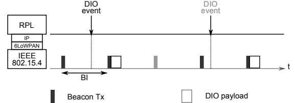
Fig. 2: Encapsulation of DIO messages in beacon frames.
