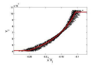
Functional relationship between reduced spectra  $\hat{b}^t X$  on the first GRSIR (PCA+ridge prior) direction and Y, the grain size of CO<sub>2</sub>.
