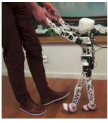
Fig. 3: Users can physically help Poppy to learn how to walk by leading it by the hands and thus providing both balance and control of mass transfer. This social guidance is also a way to make sure that Poppy will learn a human-like gait.
