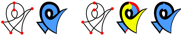
Figure 25: Left: To obtain a self-overlapping object, one “invisible edge” is necessary, to define two faces with different depth orders. Right: This ordering implies that the red edge is below the yellow face. Depending on the geometry of the invisible edge, this situation often leads to artefacts in our implementation.
