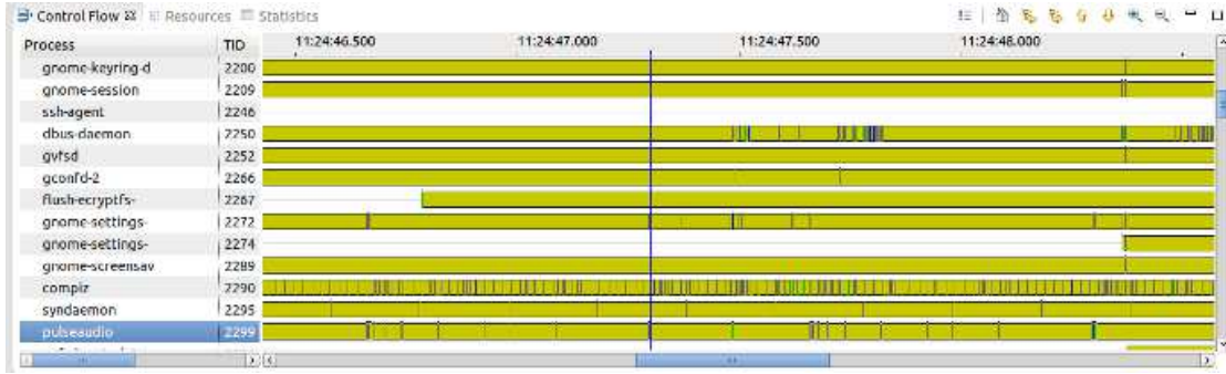
Figure 3: The LTng Eclipse Viewer [4] uses visual aggregation to avoid aliasing artifacts. However, only states that last long are easy to perceive, and an important part of the information is lost because of the aggregation
