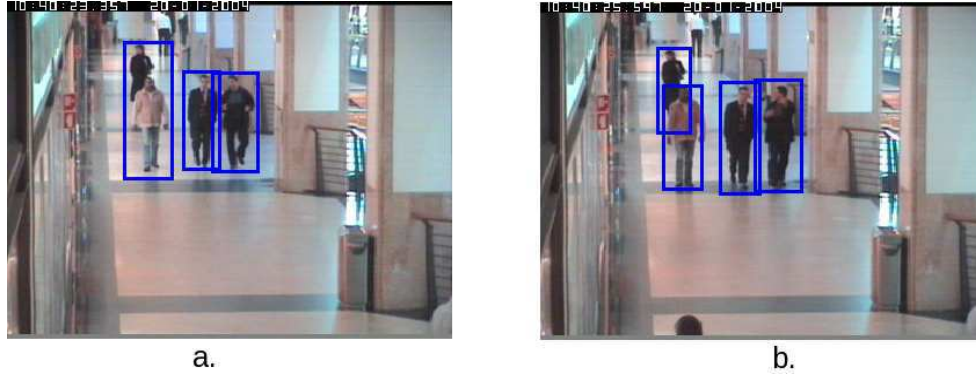
Figure 6: The influence of the object detection quality due to object location (output of [Corvee & Bremond, 2010]): a. Left image: at frame 279, the two persons on the left are wrongly detected b. Right image: at frame 335, the relative position of these two persons is changed, and they are correctly detected.
