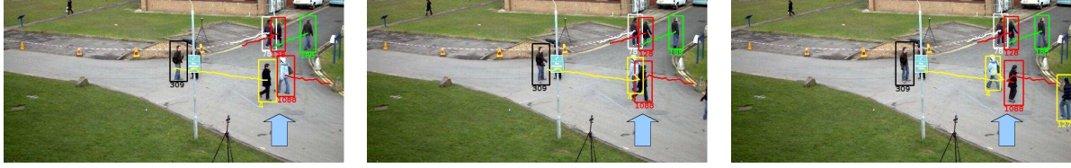
Figure 3. KLT tracker: Two persons of Id 4 and Id 1088 (marked by the cyan arrow) switch their ids after occlusion.
