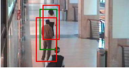
Figure 2. Illustration of the object detection correction for Caviar video. The green bounding box is the output of the object detection process. The red bounding boxes are the result of the detection correction task.
