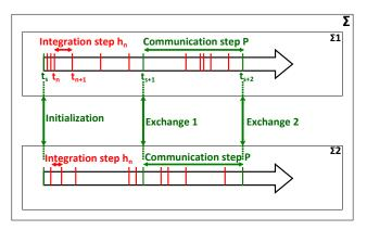
Figure 2:  $\Sigma$  split into  $\Sigma_1$  and  $\Sigma_2$  for parallel simulation.
