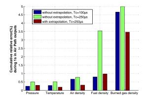
Figure 7: Cumulative relative error using different communication steps.
