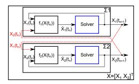
Figure 3: System's internal composition.
