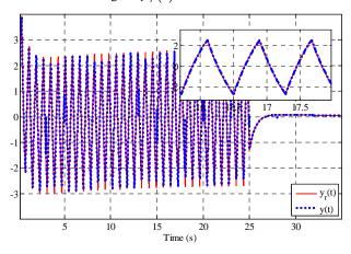
Fig. 3. Trajectory of the switched system's and the reference model's outputs.
