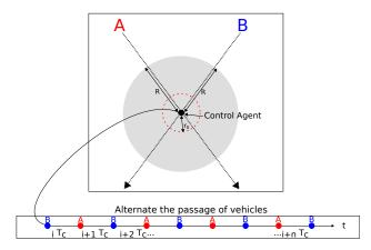
Fig. 4: Synchronization principle of an intersection
