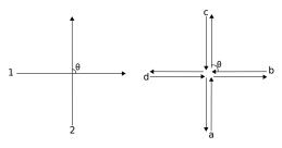
Fig. 1: Intersections with 2 flows (left) and 4 flows (right)
