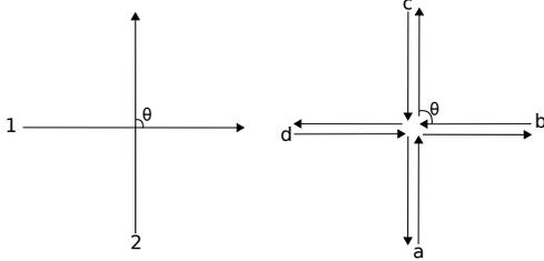
Fig. 1: Intersections with 2 flows (left) and 4 flows (right)
