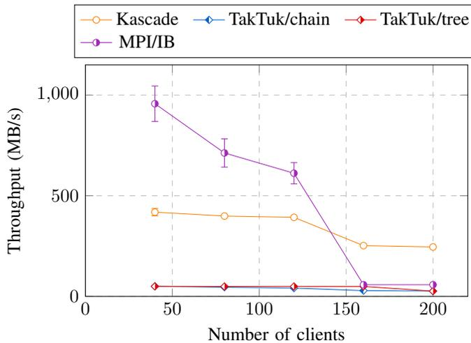
Fig. 9. The performance of the methods using IP over InfiniBand (20 Gbit/s), however *MPI/IB* is using InfiniBand directly. No method is able to saturate the bandwidth, but among them only Kascade shows scalable behavior.
