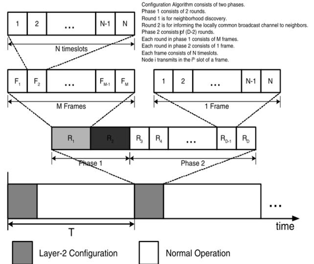
Figure 3. Operation cycle of a diameter-aware node.
