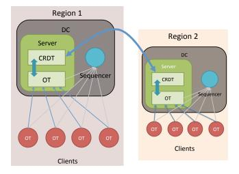
Figure 1: Hybrid deployment of the collaborative text editor.
