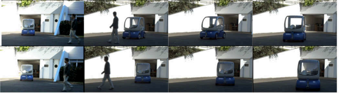
Fig. 4. Comparison between methods S (top) and M (bottom) as a pedestrian crosses the path in front of the robot.
