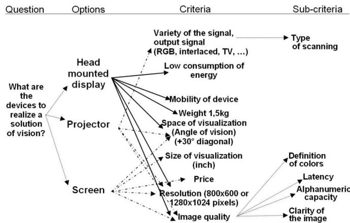
**Fig. 9.** Selection criteria for the vision support device
