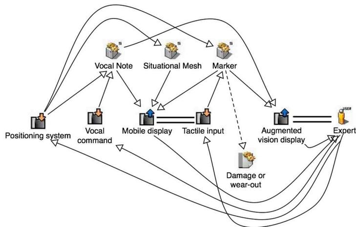
**Fig. 3.** ASUR model representing the "Create damage" task
