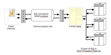
Fig. 4. The distributed architecture of HyperSmooth.
