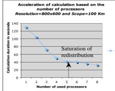
Fig. 7. Acceleration of computation depending on the number of involved processors
