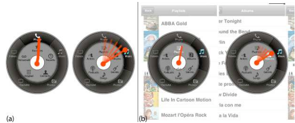
Figure 3. Previsualization using the Wavelet menu. (a) The user can browse all the submenus by performing a continuous circular gesture. (b) For consistency, the user can also browse linear lists with the same mechanism.
