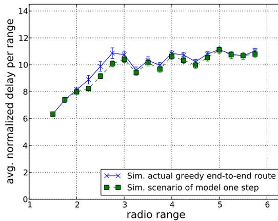
Figure 17: Normalized delay in greedy routing and model.
