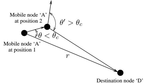
Figure 2: Figurative description of relay change due to turn. At position 1,  $\theta < \theta_c$  and node  $A$  carries the packet for node  $D$ . At position 2, node  $A$  changes its heading vector and must transmit the packet.
