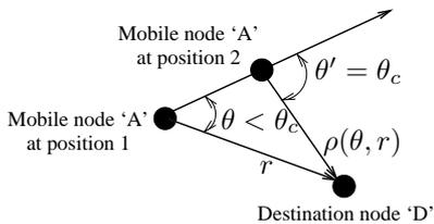
Figure 3: Figurative description of relay change due to pass over. At position 1,  $\theta < \theta_c$  and node A carries the packet for node D. At position 2, node A has the same heading vector but  $\theta' = \theta_c$  and it must transmit the packet.
