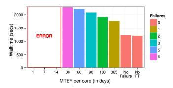
Fig. 2: Execution runtime of *Jacobi3D* application under different values of MTBF.
