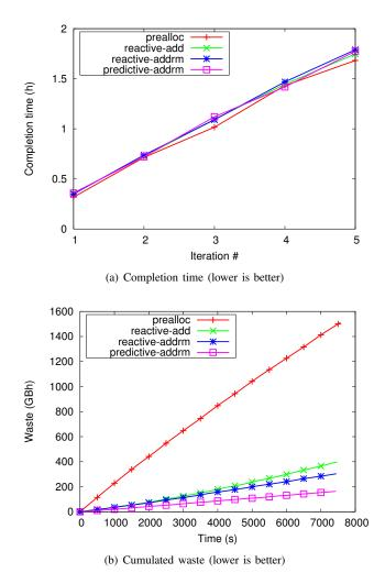
Fig. 3. K-Means: trade-off between achieved performance and waste of storage space for a Hadoop cluster made out of 30 VMs
