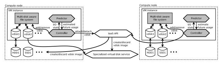
Fig. 1. Integration of our approach into an IaaS cloud architecture; components that are part of our design are highlighted with a darker background.
