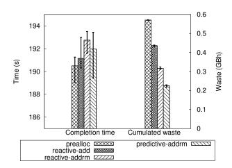
(a) Completion time and cumulated waste (lower is better, error bars represent min and max)
