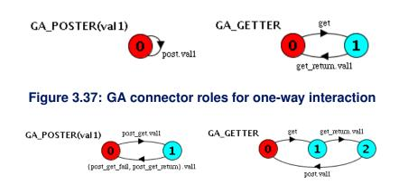
Figure 3.38: GA connector roles for two-way interaction
