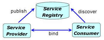
Figure 1.1: Service-oriented interaction pattern
