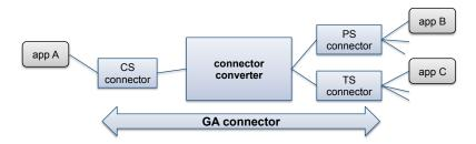
Figure 3.2: GA-based connector interoperability
