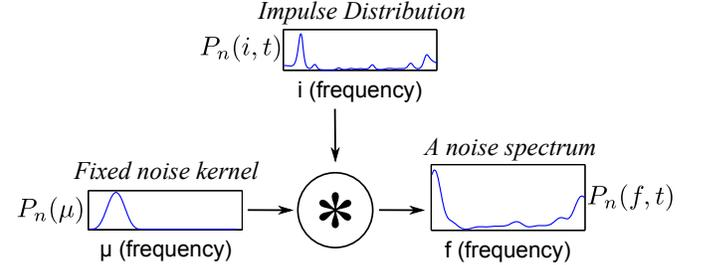
Fig. 2. Noise spectrum model
