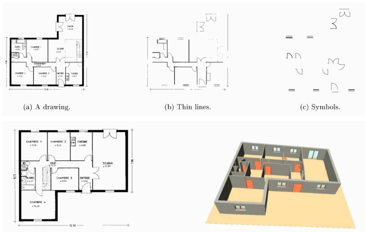
Figure 6 from [Dosch et al. 2000] representing the results at all major bottom-up stages of the interpretation process: line segmentation, symbol recognition, context identification, 3D reconstruction.
