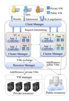
Figure 1. Architecture of Cloud Bursting PaaS System
